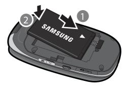
2. Press down until the battery snaps into place.
